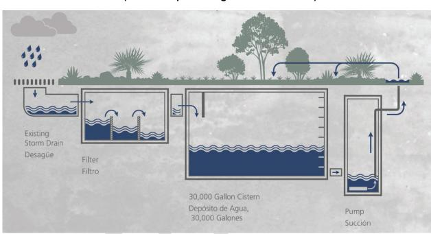
Figure 2. Stormwater capture infrastructure elements (From interpretive signs at Kimball Park)
