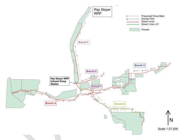
FIGURE 1 – PDMWD Sewershed, showing major sewer lines, force mains, and stormwater parcels used for volume and capacity evaluations.
